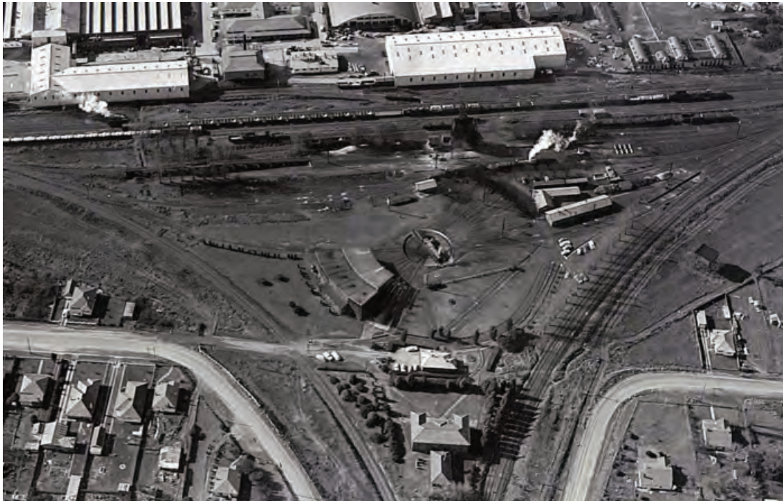
Image 2. The heart of East Fork Depot, the partial roundhouse and the turntable with its radiating 'roads'. Below the turntable is the District Locomotive Engineer's office and below that again, the barracks for visiting off-duty engine crew. Image courtesy ODHS CWD Negative Collection, photo taken 9.07.1964.
