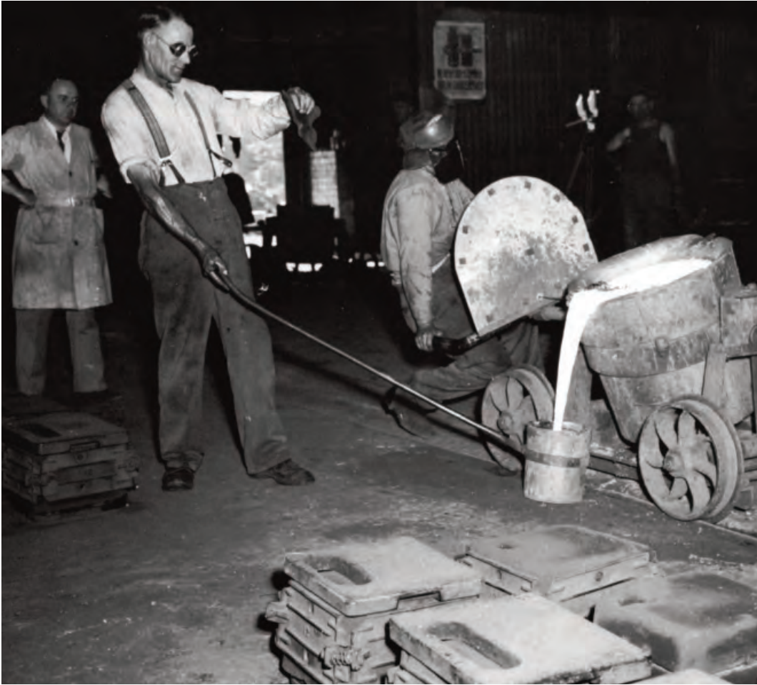
Oscar Kalms uses a long rod to steady a ladle while Bobby O'Neill pours molten iron into it from a bull ladle. The man standing in the background is supervisor Jim Brady.
